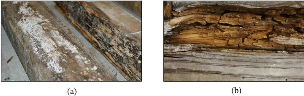
Figure 5-1 Close-up pictures of the decayed specimens: surface hyphae of the fungus (a) and internal wood damage after post-testing inspection (b)
