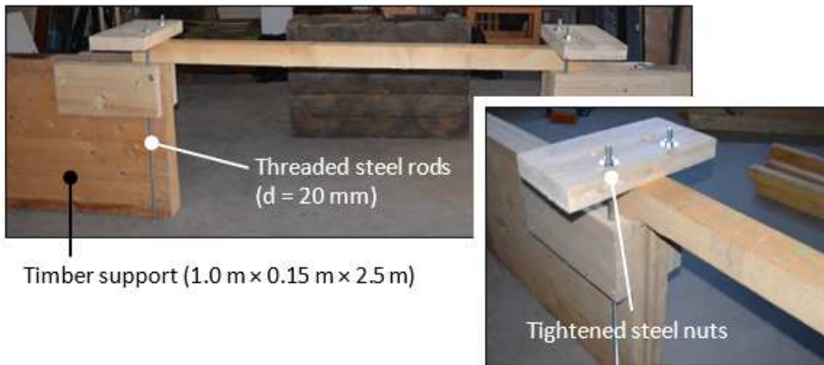
Figure 5-19 Setup adopted to replicate fixed-fixed boundary conditions: clamp apparatus between two wooden surfaces using two threaded rods with tightening nuts
