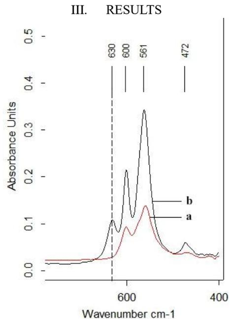
Fig. 4. IR lines for used for the evaluation of the Splitting factor. of Specimen 1 (a) and Specimen 2 (b).
