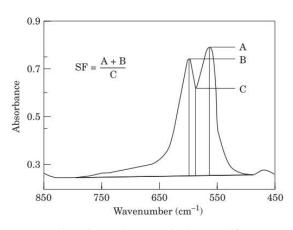
Fig. 3. Splitting factor calculation [26]
