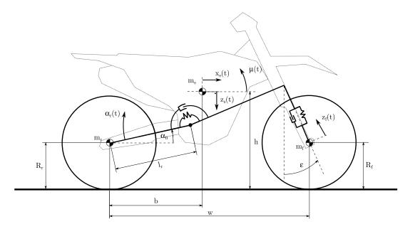
Figure 6: Five degree of freedom model of the motorcycle.  $x_s$  and  $z_s$  are the longitudinal and vertical translation of the center of gravity of the chassis,  $\mu$  its pitch rotation, and  $z_f$  and  $\alpha_r$  are the relative displacements of the front and rear suspensions, respectively.
