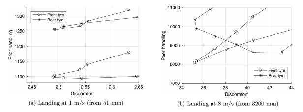
Figure 10: Handling vs comfort indices with transient excitation. The damping factor starts on 1 on the larger marker decreasing with a step of 0.05.
