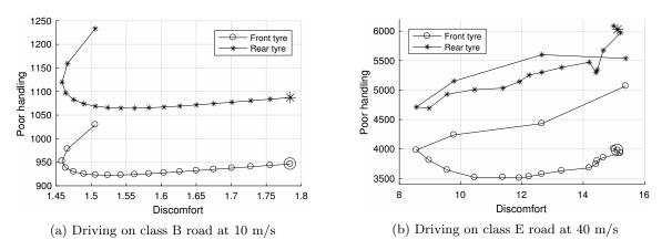
Figure 7: Handling vs comfort indices with continuos excitation. The damping factor starts on 1 on the larger marker decreasing with a step of 0.05.
