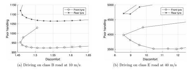
Figure 9: Handling vs comfort indices with continuos excitation. The damping factor starts on 1 on the larger marker decreasing with a step of 0.05.
