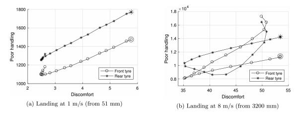
Figure 8: Handling vs comfort indices with transient excitation. The damping factor starts on 1 on the larger marker decreasing with a step of 0.05.
