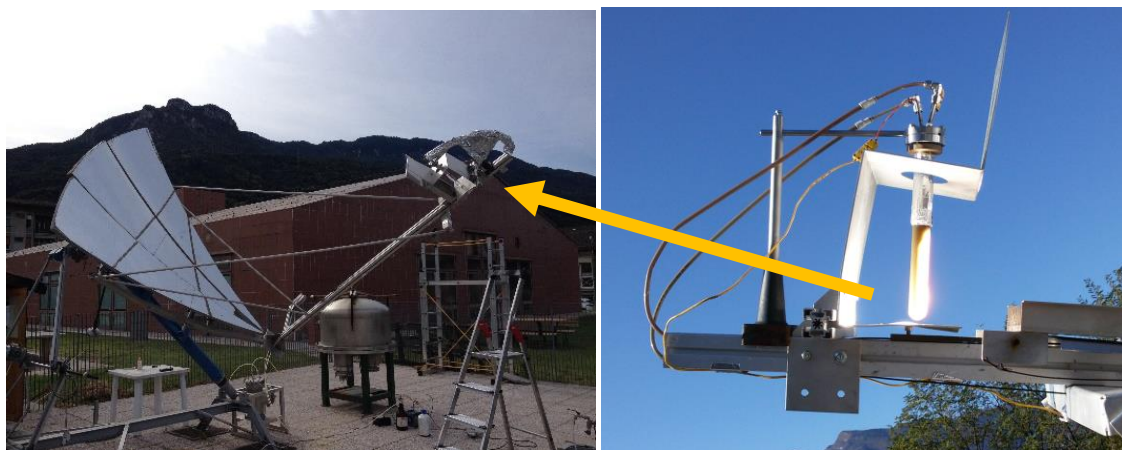
Figure 6.1: PDC configured with 3 mirror modules (left) and quartz glass lid circulating the surfactant-rich wastewater (right).
