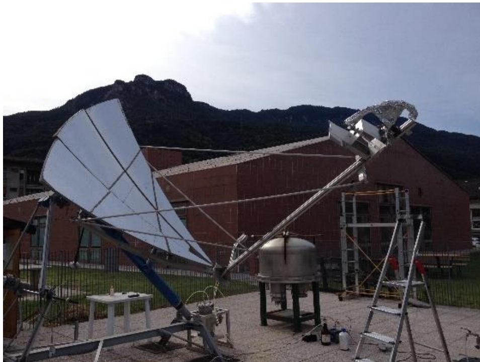
Figure 3.1: Schematic drawing (up) and an image of assembled solar concentrator apparatus (down) for experiments used in this work.
