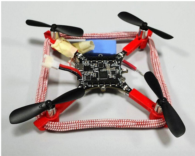
Fig. 10. Photo of the tiny drone Crazyflie with the receiving coil mounted.
