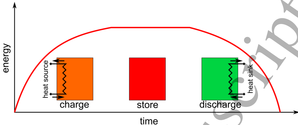
Figure 1. Typical working cycle of a TES system, showing the charging, storage and discharging steps and the variation of stored energy over time.
