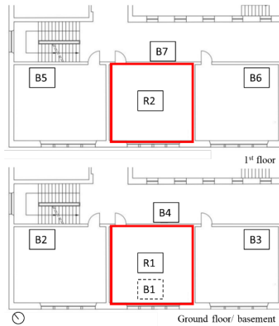
Fig. 3 – Monitoring of the case-study: sensors inside the 9 monitored rooms. Letters R and B before sensor numbering indicate respectively Reference room and Boundary room
