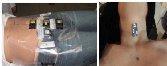
Figure 7.1: TLDs used for measuring the ESD for planning and monitoring radiotherapy treatments involving prostate (left) and thyroid (right) cancers [113].
