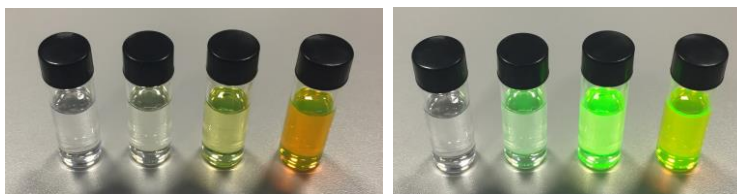
Figure 9.4: Glass vials containing toluene with dispersed CdSe/ZnS QDs at the concentrations of 0, 0.03, 0.3 and 3 mg/ml under ambient light (left) and UV light (right).
