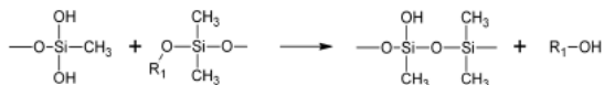
Figure 3.2: Schematic representation of the cross-linking reaction of condensation, with the formation of volatile by-products [58].
