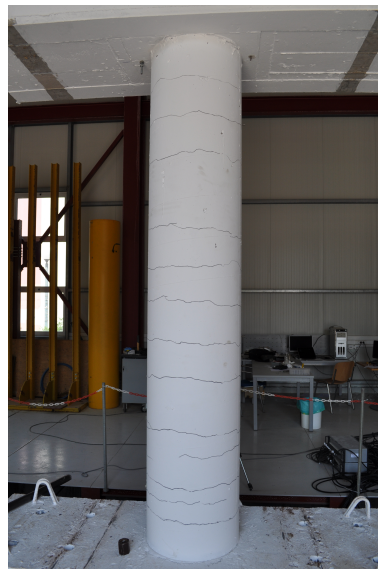
FIG. 5.92 After test 40 cm column 120%
