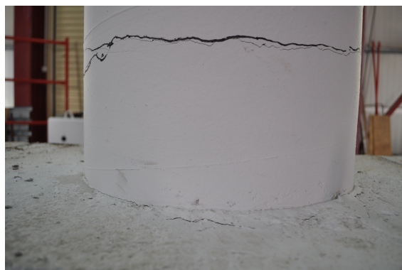
FIG. 5.93 After test 40 cm column 120%
