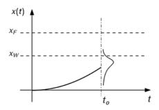
Fig. 1 is represented by a generic probability distribution. The importance of modelling the degradation of a component using a random variable is represented by the possibility to express the result using a probability that is, a degree of belief about the triggering event.
