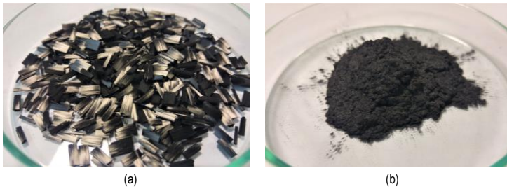
Figure III - 8. Discontinuous carbon fibers (Zoltek), as received. (a) PX35 type 65 (“long”, CFL); (b) PX35 MF150 (“short”, CFS).
