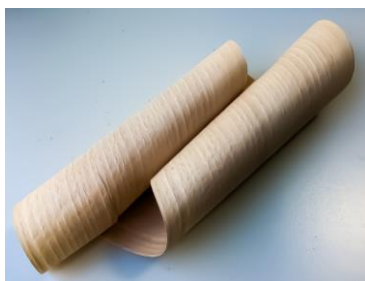
Figure III - 9. Thin beech laminae obtained at the CNR Ivalsa Institute (San Michele all'Adige, TN, Italy).
