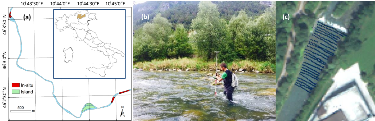
370 371 Fig. 3. In-situ measurements of water depths in (a) three reaches of the Sarca River, using (b) a RTK GPS (c) at 372 dense points along cross-sections. The location of river is highlighted in northeast Italy.
