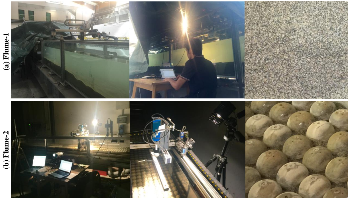
319 Fig. 1. Spectroscopic experiments in a range of water depths on (a) flume-1 with a sand bed and (b) flume-2 with a 320 gravel bed composed of semi-natural material.
