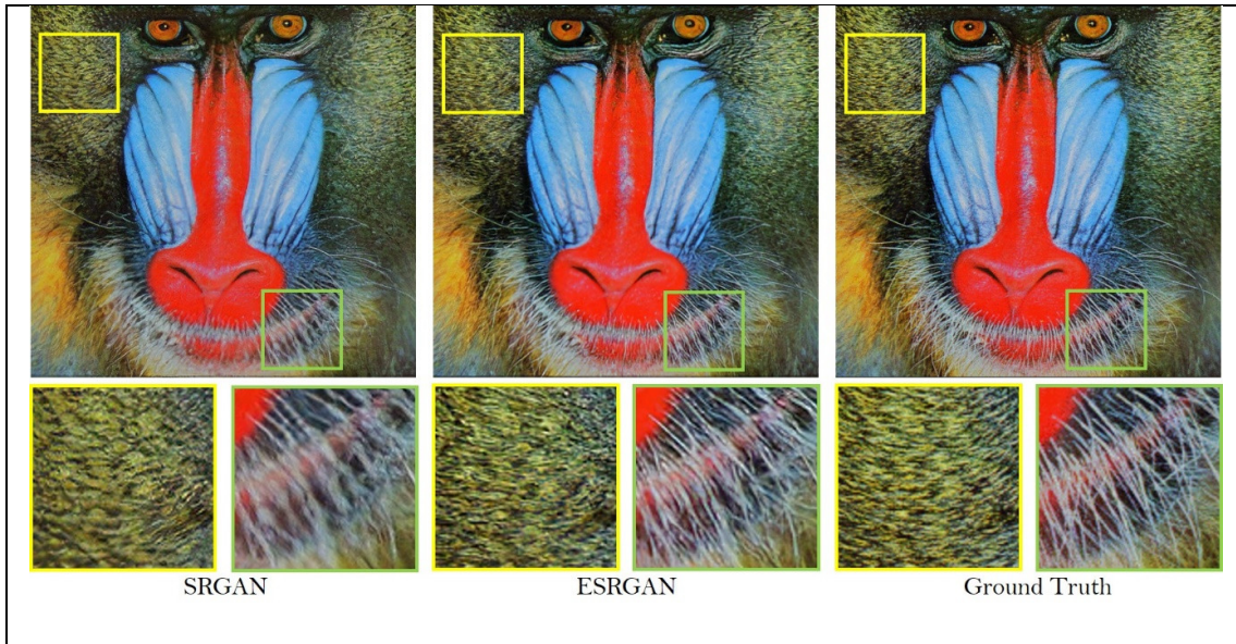
Figure 2.4 A comparison of single image super-resolution results for SRGAN and ESRGAN (Source [31]).
