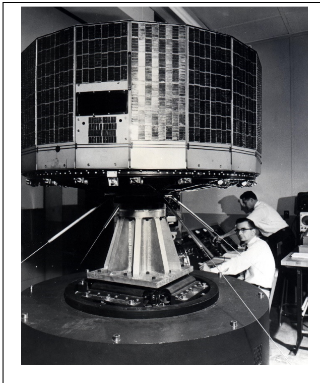
Figure 1.3. TIROS-1 the first weather satellite that demonstrated the feasibility of monitoring Earths cloud cover and waether pattern from space (source: [4]).
