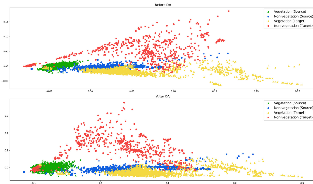
Figure 4.7 PCA distribution of source (NEWI) and target domain (NESU) test samples before (top) and after (bottom) domain adaptation.
