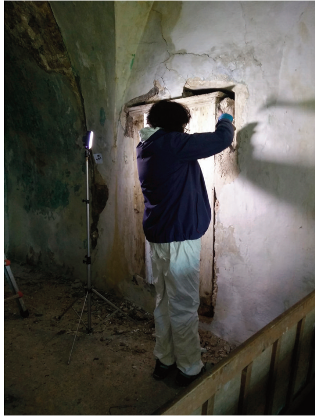
Fig. 11 | Extraction of mortar samples (credit: F. Giampiccolo, 2018).
