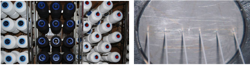
Figure 3.1: Silicone yarn bobbins produced by LeMur S.r.l. (left) and a family of six extruded silicone yarns just after the extruder (right). Pictures are taken from [1].
