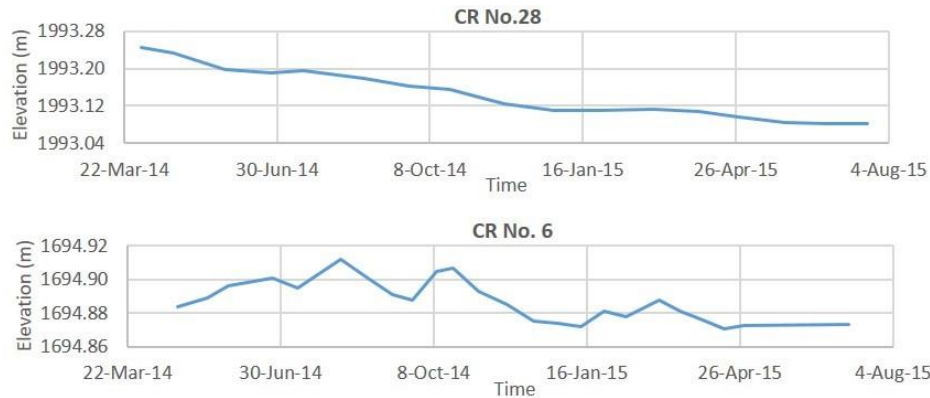
Figure 3.11 : Linear and non-linearity behaviors of CRs. Elevation changes of CR28 and CR6 are derived by the GPS measurements.
