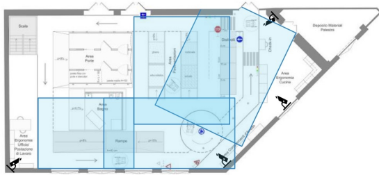
Figure 4: Layout of the AUSILIA gym. The environment is currently covered by four IP cameras, necessary to monitor the wheelchair path. The approximate coverage of the cameras is highlighted in light blue.
