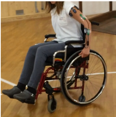
Figure 2: Image of a user testing all the described equipment: EMG sensors, electrogoniometer, and wheelchair.
