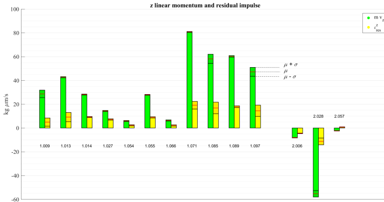
Figure 4.50: orthogonal impulse model: comparison between total z momentum and residual impulse l_{res}^z for non-compliant fast pin tests. Only reliable tests have been considered in the computation. The captions under each group of columns report the test number (e.g. 1.089 is TM1, test 89). The end of each column (of a darker colour) indicates the range of the uncertainty, as shown in the figure ( \mu is the estimated value and \sigma its standard deviation).
