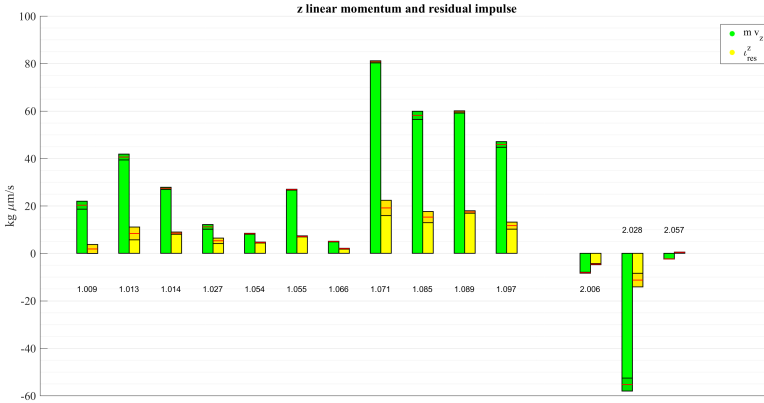
Figure 4.51: orthogonal impulse model: comparison between total z momentum and residual impulse l_{res}^z for non-compliant fast pin tests. Same result of figure 4.50, but considering (when possible for a test) a larger number of samples in the computation of the velocities.
