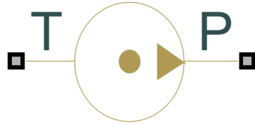
Figure A.7: Hydraulic pressure pump.
