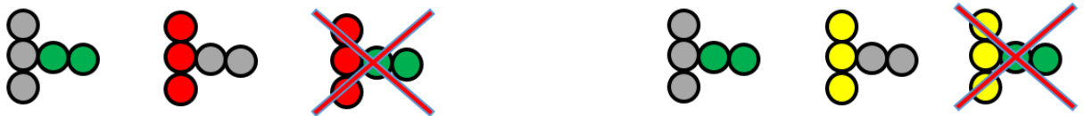
Figure 8.16: Graphical representation of the property “The two semaphore colors are always mutually exclusive”.
