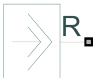
Figure A.10: Mechanical force source.
