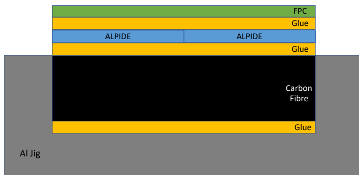
Figure 3.23: Stratigraphy of DUT. Different layers are not in scale.
