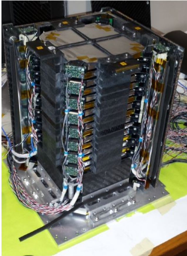
Figure 1.10: Calorimeter of HEPD-01 detector [15].
