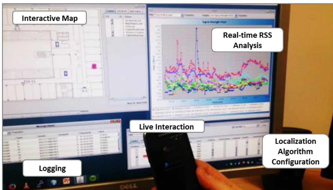
Figure 12. Graphical user interface of the wireless localization system providing the “location-based” features of the monitored users.
