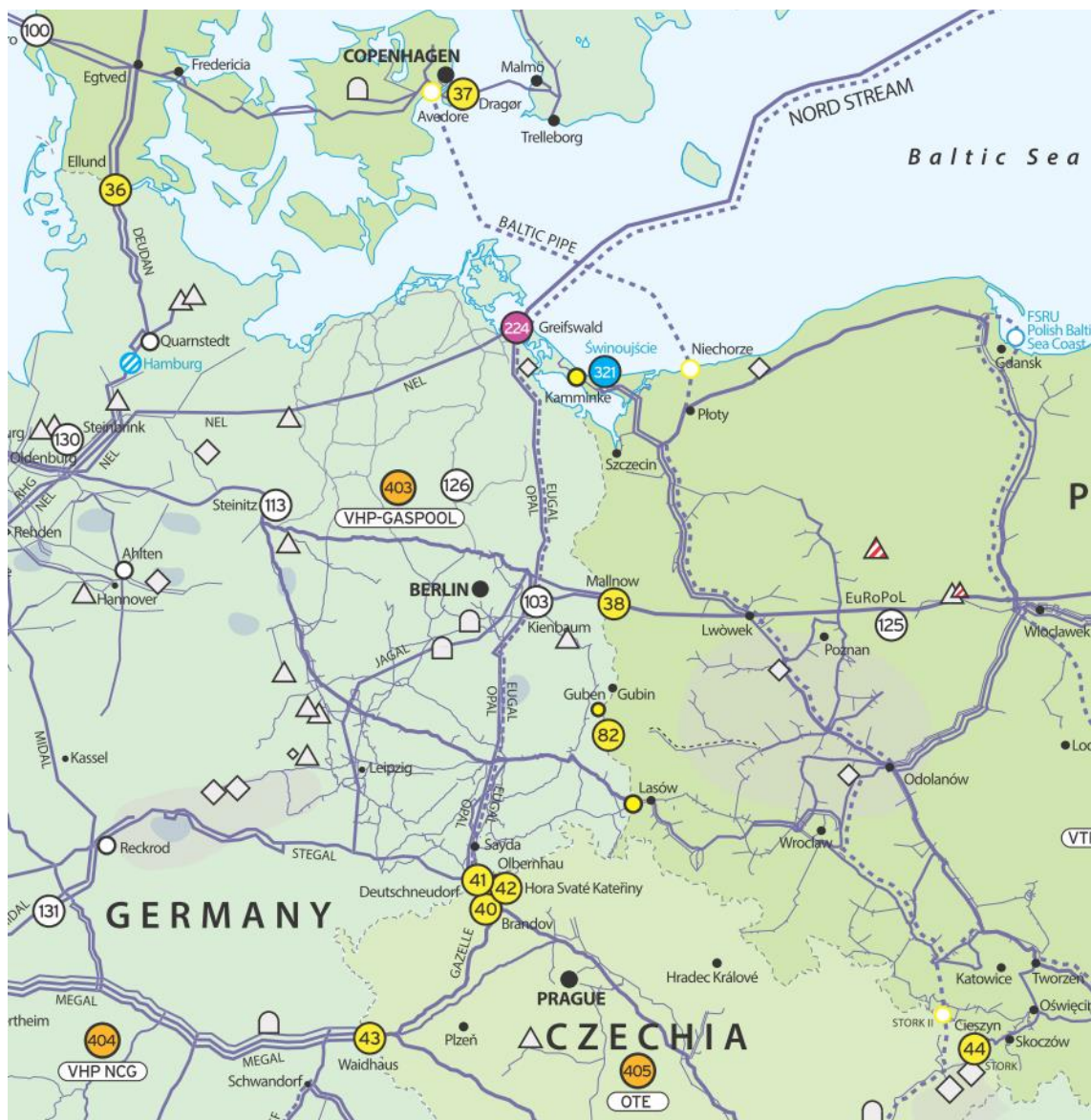
Figure 4: The OPAL pipeline delivers Russian natural gas from the north to the south, with the entry point at German Greifswald and the exit point at Brandov in Czechia.
