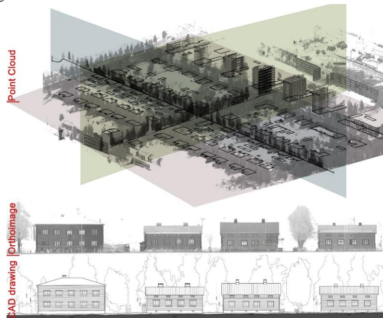
Fig 3. The process of redrawing the laser scanning survey. By exporting Ortho-images it is possible to elaborate the CAD drawings. The point cloud can be updated and used for monitoring specific situations over time.
