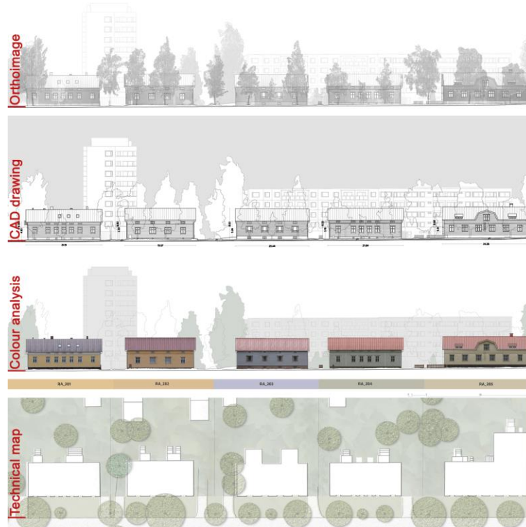
Fig 5. Extract of digital documentation elaborated for the whole neighbourhood of Raksila, technical drawings, photomaps, dimensional analysis.
