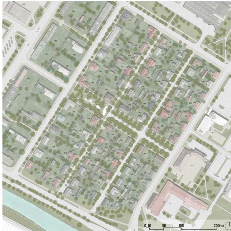
Fig 4. The map of Raksila updated on the base of the point cloud. The map includes all different levels of information, from the measures to the characteristics of buildings, streets and vegetation.
