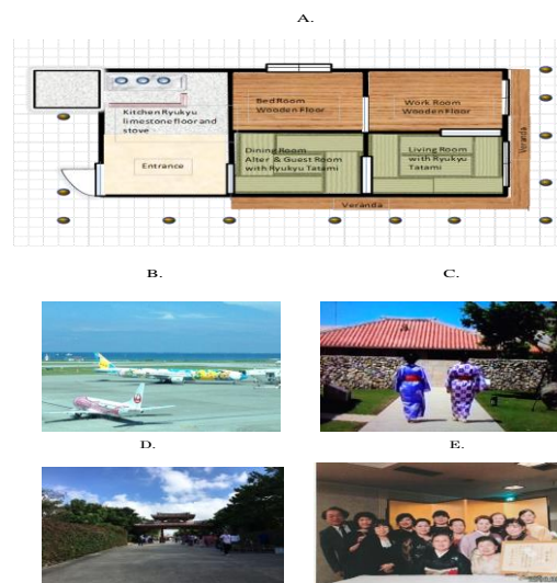
Figure 3 [(A) The following is the floorplan image (Sources: Okinawa Prefectural Museum and Art Museum plaque, [30][31] re-sketched into English for the reader to see and understand. The kitchen stove and floor material is Ryukyu lime stone. The entrance floor material is the natural ground itself. The bed room, work room, and veranda floor was made of Fukugi wood. The Dining and Living room floors have Ryukyu Tatami floor mats which are different from Japanese Tatami. Ryukyu Tatami is 880centimeters x 880centimeters whereas Japanese Edo (Tokyo) Tatami is 176centimeters x 88centimeters, Kyoto Tatami is 191centimeters x 95.5centimeters in comparison [32] . Japanese Tatami (Edo and Kyoto) have borderlines so that samurai wouldn't get attacked from the bottom with swords. Ryukyu Tatami culture shows that Ryukyu lived in tolerance of disasters. The concept is the equivalence of Karate (empty hand) for defence. The author used the Japanese Tatami as an image below to show the reader the comparison of "borderless" between Ryukyu and Japanese Tatami as well as a metaphor. (Translated into English and re-sketched using Excel by Hirona Matayoshi): [(B), (C), (D), and (E): [(B) Naha International Airport and the sapphire blue sky and ocean. (C) Traditional Ryukyuan House with traditional Ryukyuan Kimono Chignon hairstyles and the Karaji Yui. (D) Shuri Castle Gate. (E) Masters with their award (The location was in the Okinawa Prefectural Museum and Art Museum) (Source: Photographed by Hirona Matayoshi .)]
