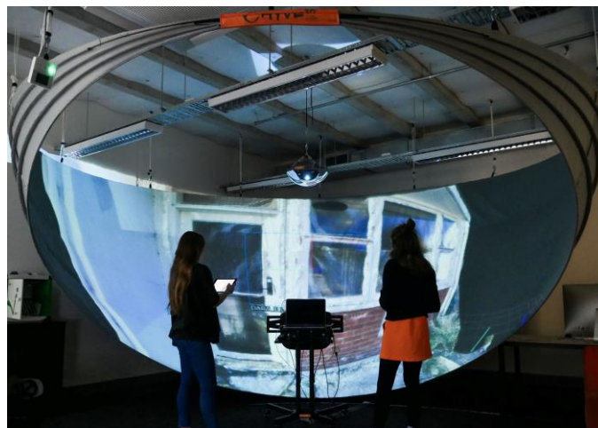
Figure 5. The Hyve3D social immersion in use; virtual model is projected onto a concave surface, immersing the users within it.
