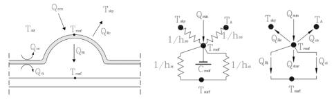
Fig. 5. Heat balance and RC scheme for the heat transfer process.
