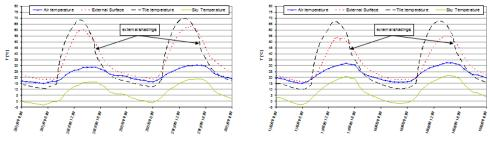
Fig 6 Temperature measured and simulated for roof A (left) and B (right).
