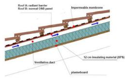
Fig. 1. Cross section of the two roof analyzed
