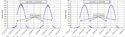
Fig. 2. Solar radiation on tilted surface for roof A (left) and for roof B (right).
