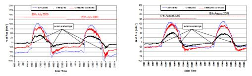
Figure 7 Trend in external heat flux for roof A (left) and B (right).
