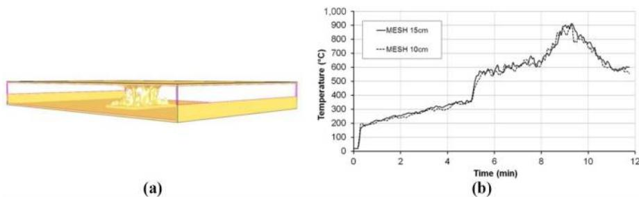
**Notes:** (a) Fire development modelling; (b) temperature development at the ceiling level with different mesh grids owing to a Class 3 three-car time-shifted fire
