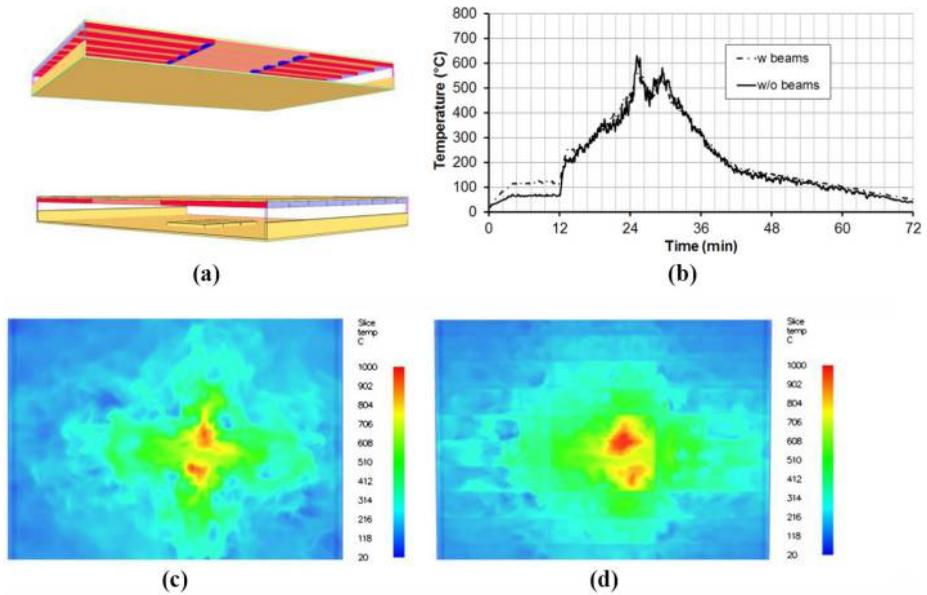
**Notes:** (a) Compartment modelling with beams included in the CFD model; (b) gas temperature evolution around the top of the HEB220 column without (w/o) and with (w) beams included in the CFD model; (c) gas temperature distribution at ceiling level at 30min without including beams; (d) gas temperature distribution at the ceiling level at 30 min, including beams
