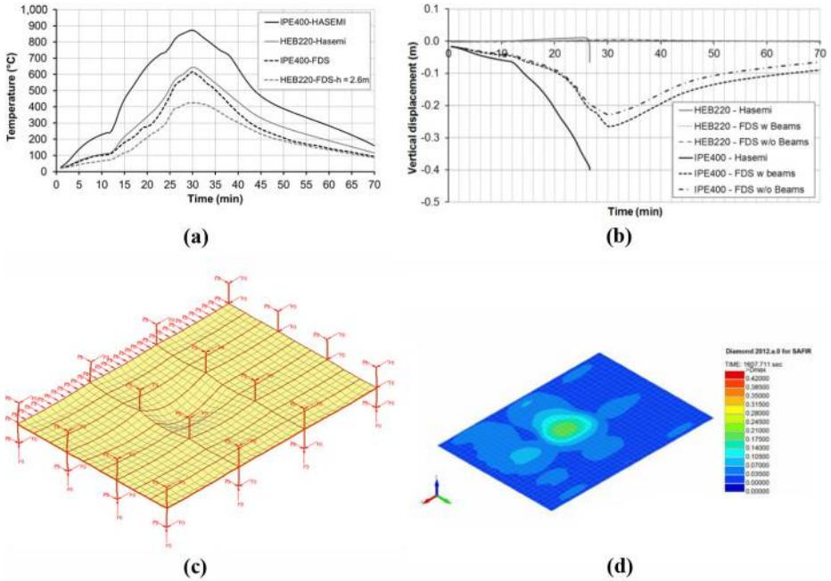
**Notes:** (a) Comparison of the temperature evolution in the web of critical sections of the column (HEB220) and of the secondary beam (IPE400), CFD model w/o beams; (b) comparison of the mechanical response of the critical sections of the column (HEB220) and of the secondary beam (IPE400); (c) deformed shape at 27 min amplified by a factor of 10; (d) vertical displacements at 27 min
