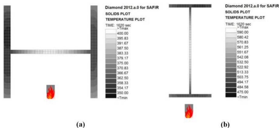
**Notes:** CFD model w/o beams; temperature distribution at 27 min in the critical section: (a) of the column (HEB220) and; (b) of the secondary beam (IPE400)
