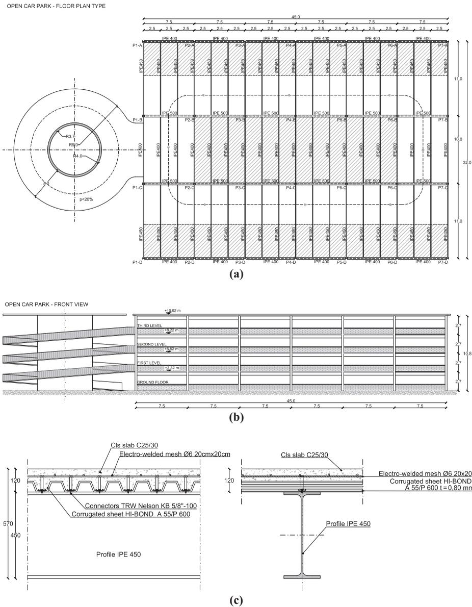
**Notes:** (a) Plan view, dimension in m; (b) elevation view, dimension in m; (c) detail of the composite slab, dimension in mm
