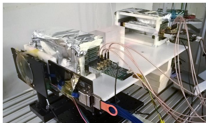
Figure 13. Picture of the setup used at the APSS proton beamline. From the left: the ALPIDE chip independently tested, one calorimeter station, the beam absorber and finally the second calorimeter station.
