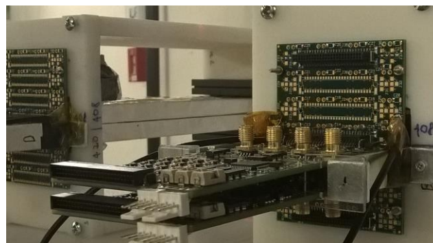
Figure 12. Detail of the tested two-module arrangement: front-end electronics in front and scintillator fingers on the foreground/right. Numbers marking the scintillator type (BC-408 and BC-420) are visible
