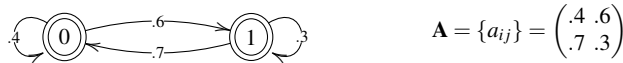
Fig. 1 A graph showing a first-order, 2-state Markov chain and its transition probability matrix \mathbf{A} . The states are labeled as “0” and “1” and the arrows represent the transition probabilities.
