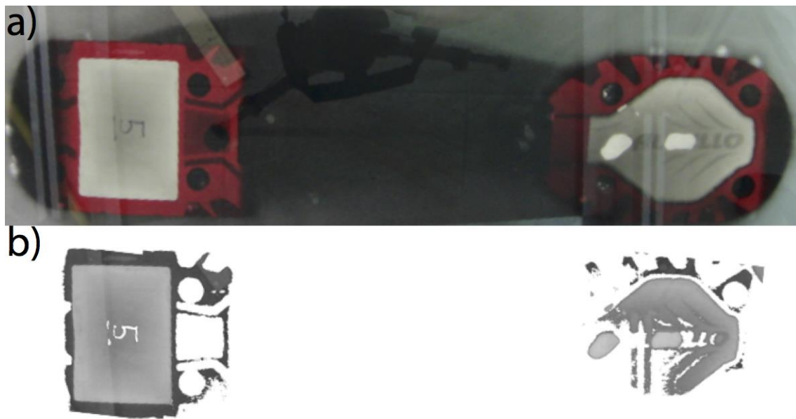
Figure 2. Images of the Sole 1 acquired with a Casio~Exilim~EX-FH25 digital camera with resolution of 3648x2736 pixels. (a) Sole with contrast liquid; (b) surface in contact.
