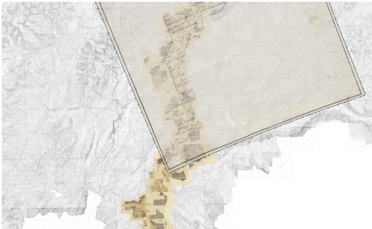
Figure 6. Detail of the Index-map of the Nowack-Plan reprojected in ETRS89, overlaid on sample map-sheets of Austrian Cadastre (ETRS89) and on Official Topographic Base Map (CTP) of the Trento Province. Source: courtesy from Cadastre Service-Autonomous Province of Trento (Italy) and Tiroler Landesarchiv (Innsbruck); adapted by the authors.
