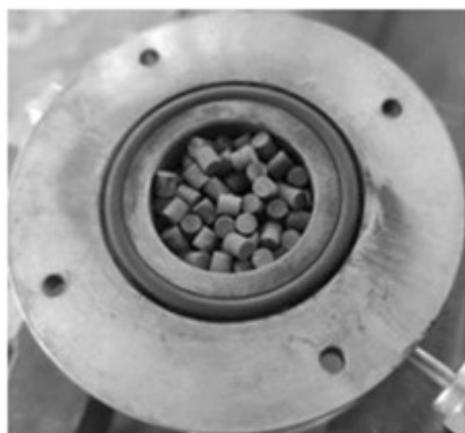
Figure 1. Catalytic chamber filled of commercial Pd/ Al_2O_3 pellets. Reproduced from [81] with permission under OA Creative Commons Attribution-Non Commercial 4.0 International License (CC BY-NC 4.0).
