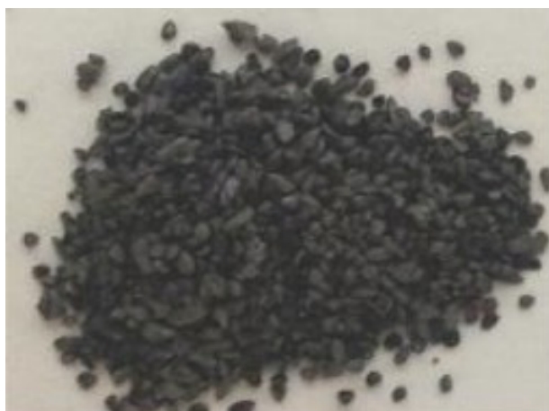
Figure 6. S405 catalyst (30% Ir/ \text{Al}_2\text{O}_3 ) [110]. Reprinted from Ref. [110] with permission from Elsevier.
