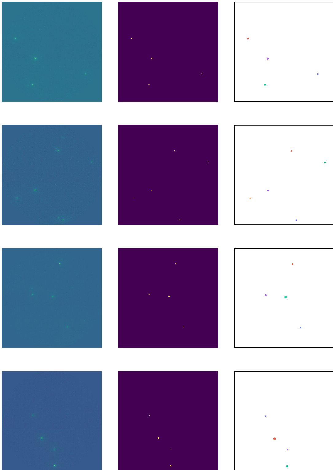
Figure 5.30 – Series of MCP pictures to show the results of the HDBSCAN clustering algorithm: on the left the original images are shown, in the centre the result of the filtering is displayed (binarisation threshold = 0.4, kernel-size = 5), and on the right the corresponding clusters identified is presented.
