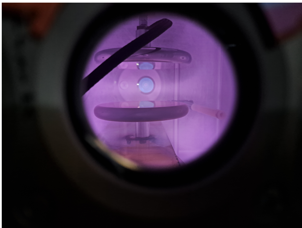
Figure A.4: Discharge in pure hydrogen at 0.05 mbar in plate-to-plate configuration, showing a diffuse glow across the electrode gap at very low pressure.
