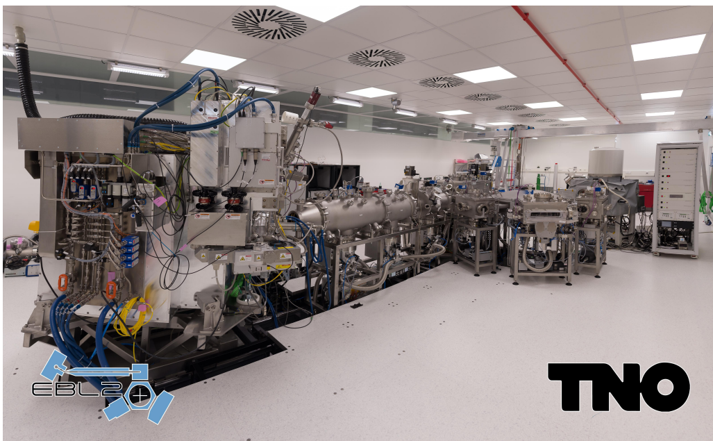
Figure B.2: Photograph of the EBL2 system corresponding to the schematic in Fig. B.1, from left to right: EUV source, collector module, exposure chamber, vacuum handler with load lock, storage, and XPS. The atmospheric handler with pod opener is not yet present. Reproduced from [53].
