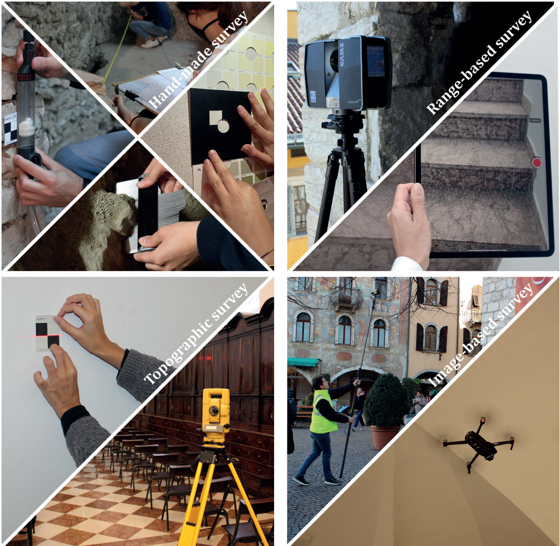
Fig. 4.10 Left, some traditional methods: hand-made survey and topographic survey; right, some digital methods: range-based survey (i.e. Terrestrial Laser Scanner, tablet with LIDAR sensor).
