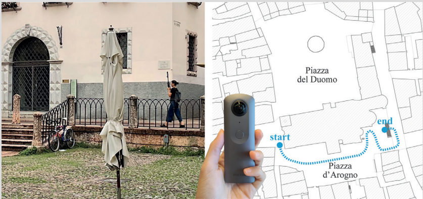
Fig. 4.24 Digital survey campaign in August 2023: the current state of the square and the staircase were recorded in a spherical video with the Ricoh Theta V 360° camera, following the blue path in the figure.
