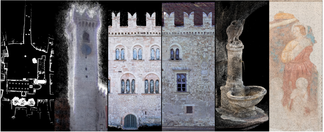
Fig. 4.3 An evocative image showing the amount of data acquired using different 3D digital survey technologies. From left to right: mobile laser scanner, spherical camera, camera on a telescopic rod, terrestrial laser scanner, tablet with a LIDAR sensor, and drone.
