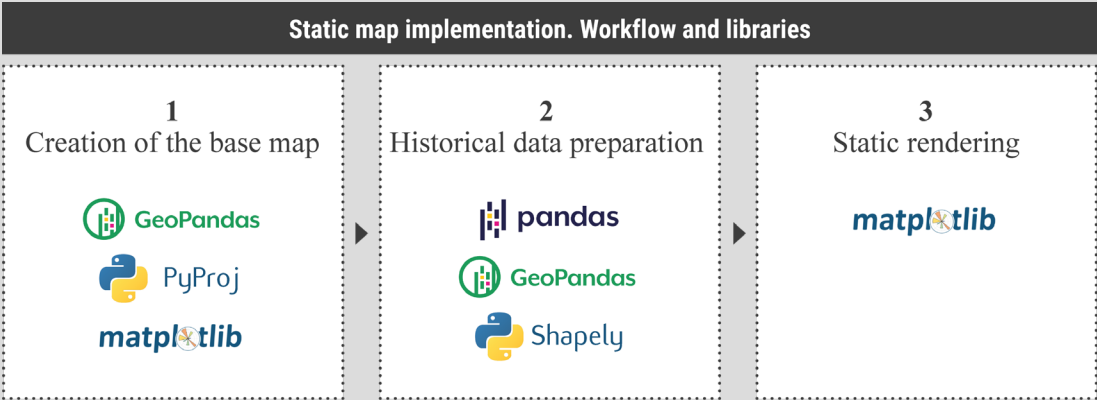
Fig. 3.21 The main steps in developing the base map and the Python libraries employed at each stage.
