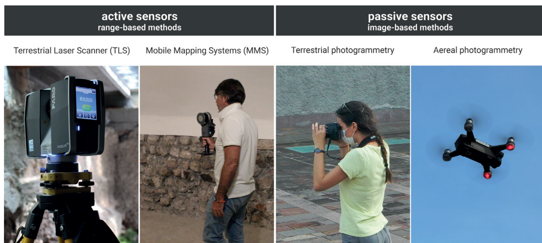
Fig. 4.8 Some of the main range-based and image-based tools used in the field of architectural survey.
