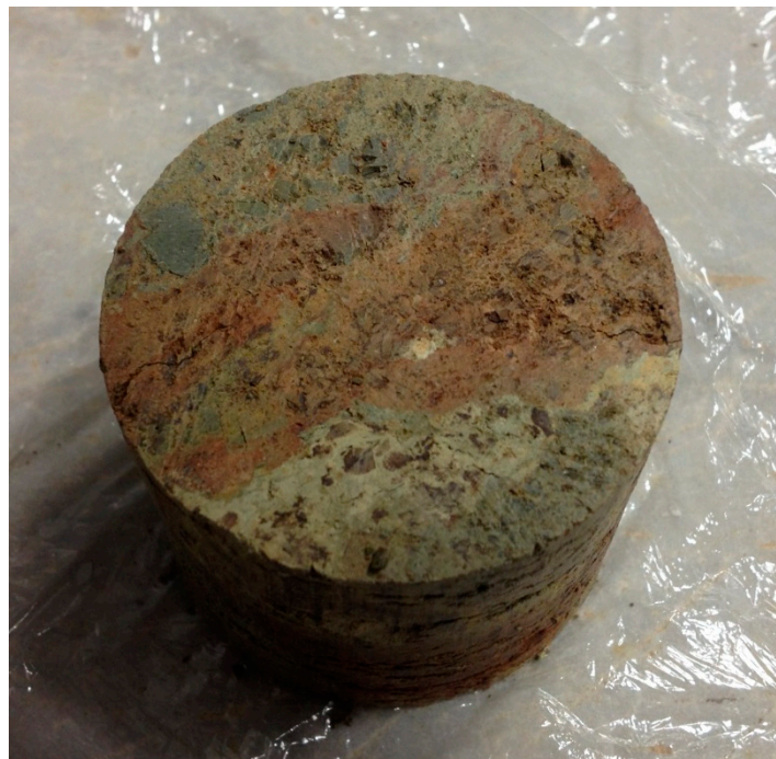
Figure 3. Specimen prepared for suction measurements (50 mm diameter, 40 mm height).
