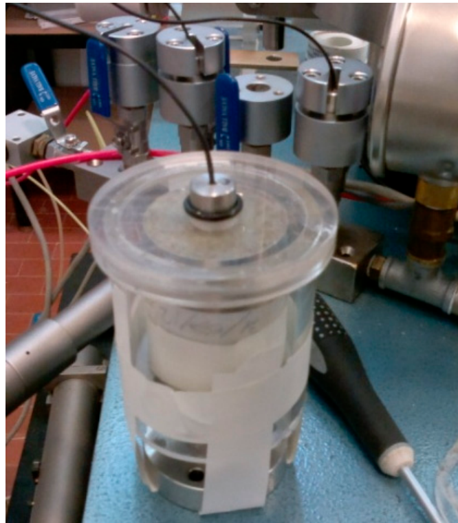
Figure 4. Example of high-capacity tensiometer measurement.
