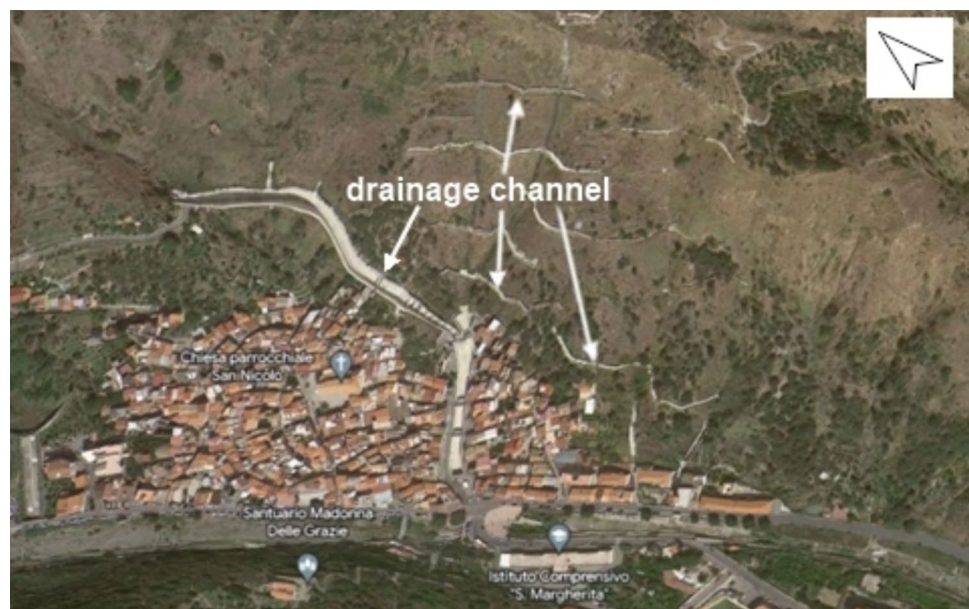
Fig. 6 The new settlement of the Giampilieri's territory with the main and secondary drainage channels
