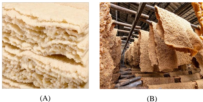
Figure 2.35. The two categories of creep rubber. (A) Pale Latex Crepe and (B) Estate Brown Crepe [108,109].
