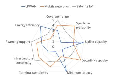
Fig. 3. Radar chart to compare the envisioned KPIs across different longrange IoT technologies (LPWANs, mobile networks, and satellite IoT).
