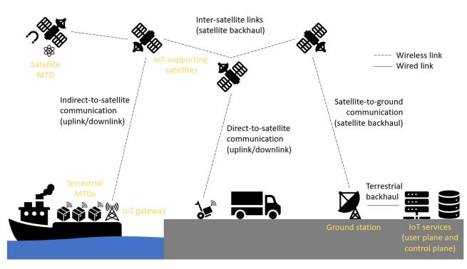
Fig. 2. Reference architecture of a satellite IoT systems. The infrastructure components are labeled in yellow, while the communication architecture components are labeled in black.
