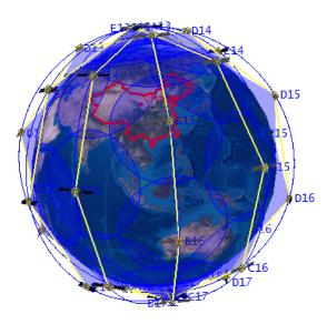
Fig. 6. Example of 3D coverage diagram of LEO constellation for IoT, with inter-satellite link (courtesy of [41]).
