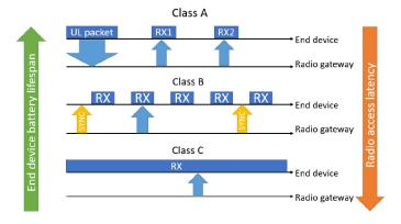
Fig. 1. Graphical description of the three LoRaWAN classes.
