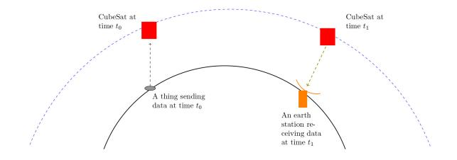
Fig. 8. Representation of typical Lacuna Space time displacement between uplink and downlink.
