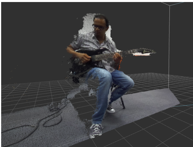
Figure 3: Example of a point cloud captured by the ZED camera during a live performance
