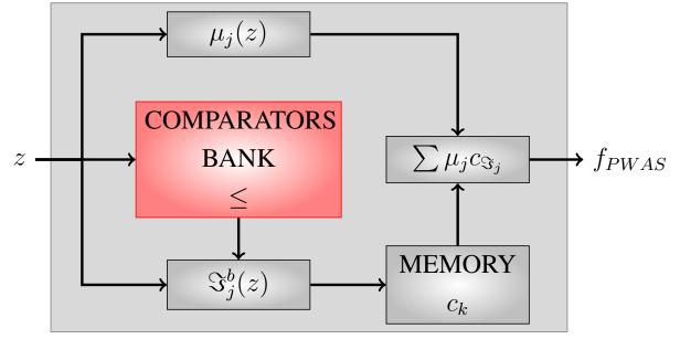
Figure 3.3: Architecture to implement discontinuous functions
