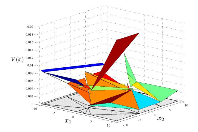
Figure 4.2: The PWA Lyapunov function for the extended system in case A
