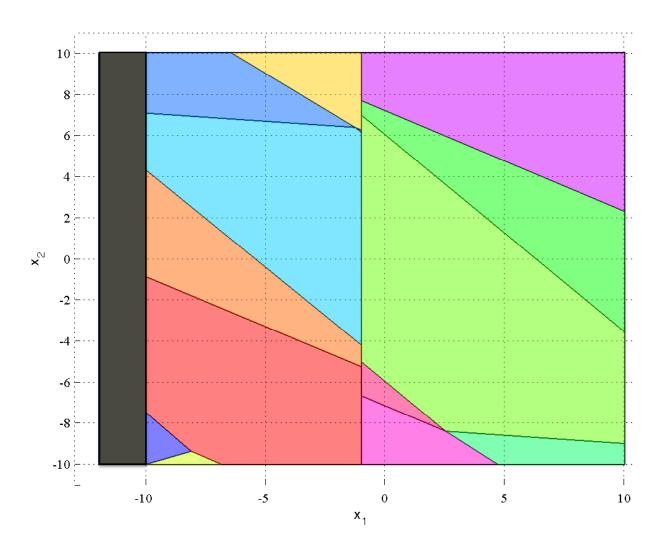
Figure 4.1: The invariant set  $\mathcal{X}_H$  for case A is constituted by the union of the regions of the explicit MPC and the box  $\mathcal{X}_H \setminus \mathcal{X}$  (the grey rectangle on the left)
