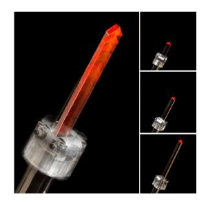
Figure 1.7: Left: a dynamic photo showing the torsional 'gun' in action; if the system is quickly twisted, the release mechanism of torsional elastic energy produces a propulsive force. Right: a sequence of three photos taken at 30 fps, showing that the propulsive force overcomes gravity.
