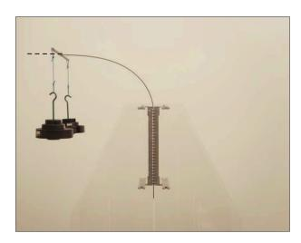
Figure 5.6: The vertical and upward Eshelby-like force (equal and opposite to the applied downward load) generated by the sliding sleeve makes the equilibrium configuration possible, even if unstable. Note that the tangent to the end of the blade is horizontal, as will be theoretically rationalized in the next section.
