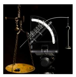
Figure 1.5: Scales across millenia: a traditional balance (left) is based on the lever principle, while the innovative elastica arm scale (right) is based on deformation and principles from configurational mechanics. In this particular configuration, the deformable arm scale is working without counterweight.
