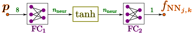
FIGURE 4. Internal structure of the neural networks f_{\text{NN}_{j,q}}(\mathbf{p}) , j \in [1, 2] , q \in [1, 2, \dots, D-2] , providing the neuralized polynomial terms in (8)-(9). The numbers in green indicate the size of the propagated signals.
