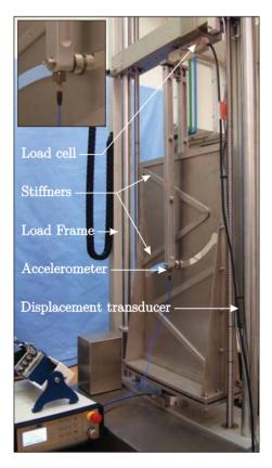
Fig. 2.20: The experimental set-up for the buckling tests, seen from the back.
