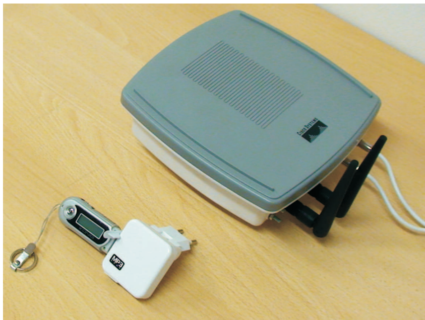
Figure 4.2: FM transmitter and Wi-Fi access point.
