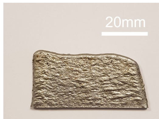
Fig. 6 Direct Laser Deposition of H13 single walls with ZigZag strategy.
