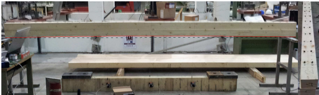
Fig. 7.3 Composite beam C1 after fastener insertion (starting from the beam centre)
