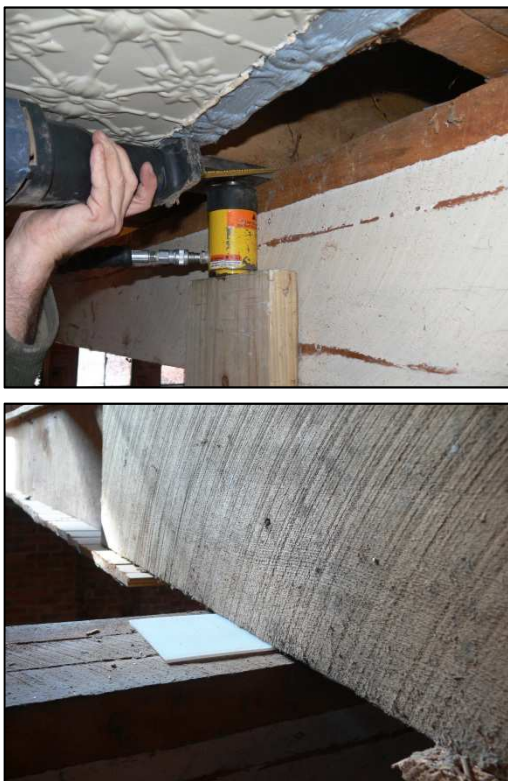
Fig. 5.4 Isolation of the specimens: a) nail cut; b) insertion of the low-friction sheets.
