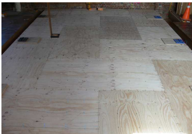
Fig. 5.20 Specimen B: plywood panel disposition
