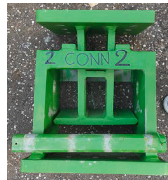
Fig. 17. SD - Pin Extraction after SD test.
