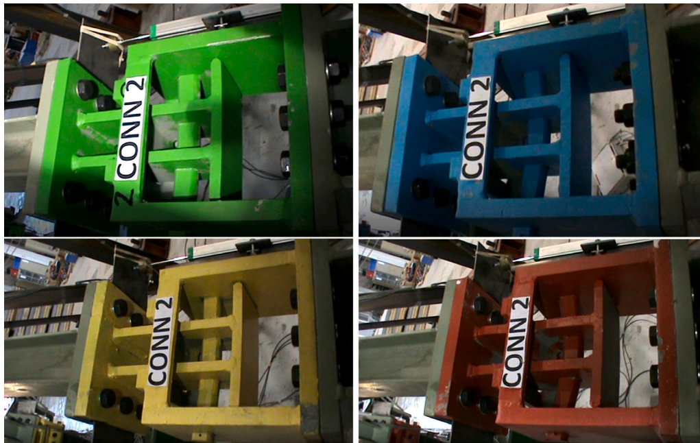
Fig. 25. DRBrC component number 2 during peak response at SD and NC limit states, for both mild steel and HSS components.
