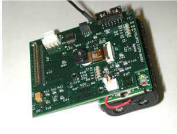
Figure 6. Cyclops couples with a Berkeley Mote and they represent a wireless vision network node.
