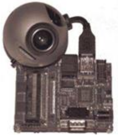
Figure 3. Panoptes, smart camera mote architecture hardware and power consumption
