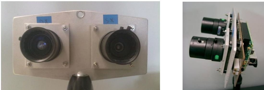
Figure 43. First Stereo prototype
