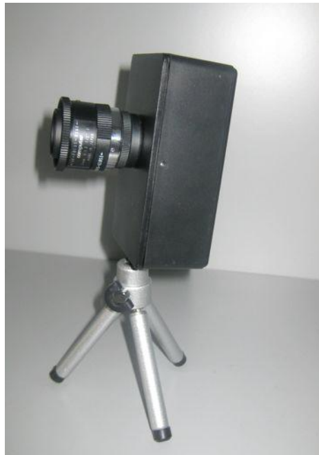
Figure 57. The prototype realized on FPGA platform usb link with a PC
