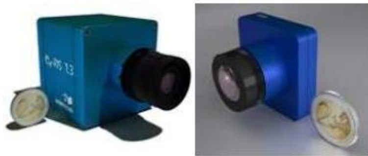
Figure 10. Eye-RIS v1.3 and v2.1 vision system.
