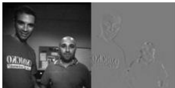
Figure 12. Sampled intensity from the Temporal difference about Etienne-Cummings sensor.
