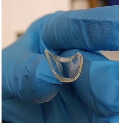
FIGURE 4.10: Flexible PSS sample obtained after UV curing.
