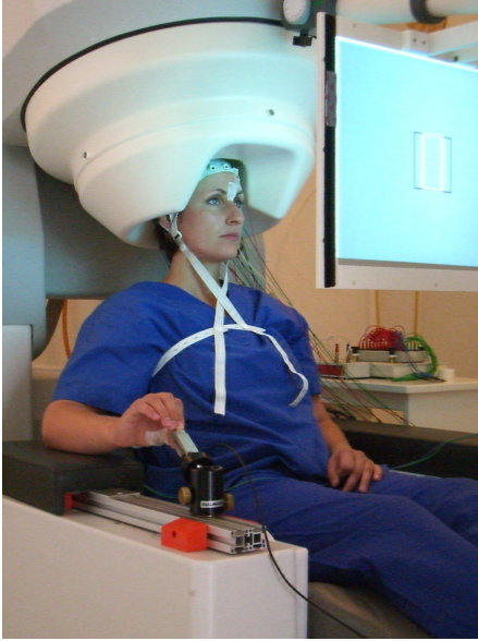
Figure 3.1: Experimental set up. The subject sits inside the magnetically shielded room with the helmet shaped dewar, with the EEG cap on the head. The screen in front of the subject displays the feedback and the fixation cross. The pinch grip is on the subject's right side.
