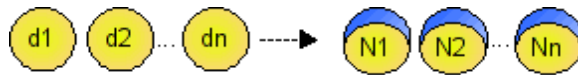
Fig. 2. Conversion of data units into SKOnodes, the light blue portion of each node represents the metadata of the node while the bottom yellow part represents its data.
